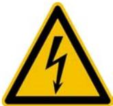
The whole circuit including the attached components (e. g. the LEDs) and wires may show up to 350V peak voltage referred to ground. **Please do not touch the circuit and the connected components including the LEDs** if the circuit is powered up. In case of failure please switch off or separate from mains voltage immediately. Do not try to repair the module even it seems simple; this includes also broken fuses.
