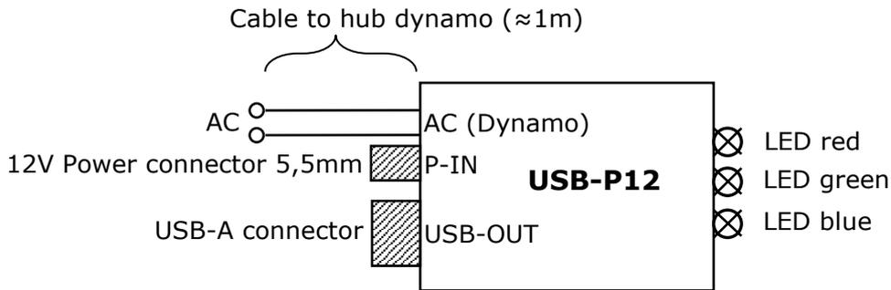
AC: input, connection to hub dynamo, two-core cable, 1m, black, fixed to box
