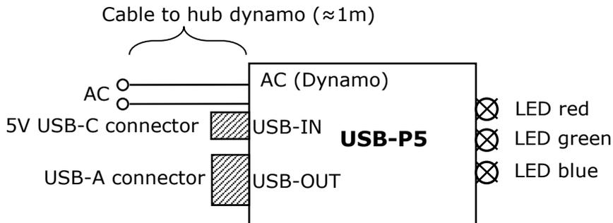
AC: input, connection to hub dynamo, two-core cable, 1m, black, fixed to harvester
